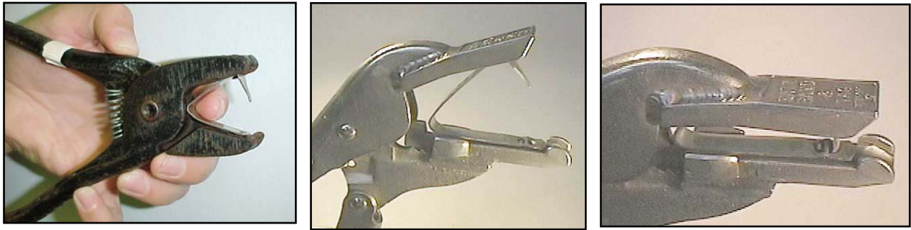
Figure 8. A Monel 1005-49 style metal flipper tag correctly loaded (left) and cinched (right) in the application pliers. ALWAYS align the base plate of the tag flat against the pliers. Note the tine bent over and completely through the stirrup. Source: http://www.nationalband.com/nbt.pdf
