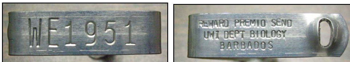
Figure 3. Enlarged view of the dorsal (alphanumeric) and ventral (return address) faces of an Inconel 1005-681 tag available from the Marine Turtle Tagging Centre (MTTC). Photo: Stacy Kubis/ WIDECAST.
