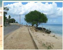
Solid coastal structures like boundary walls and fences, curbs and roads can prevent beaches from forming
